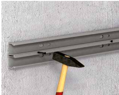
WDK with nail strip The nail strip means that WDK trunking can be mounted with steel nails. At the same time, it prevents nail damage to the cables. Of course, the nail strip can also be used as a separating retainer for routing different voltage levels.
