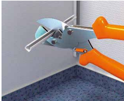
Cutting mini trunking The OBO shears can be used to create an exact straight cut for the WDK trunking. The shears can be used for trunking sizes of up to 25 x 45 mm.
