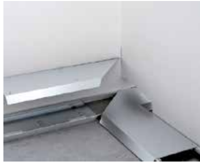
T piece With the T piece, the trunking base is not needed in the width of the junction trunking, whereas the rear side profile must completely bridge the reverse interruption. The junction trunking (AIK-F.), with the one-sided slope, is covered using internal corner lids.
