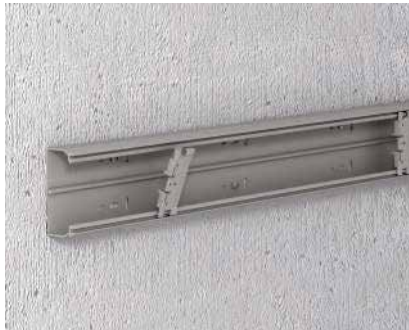
Cover clip mounting The cover clip is locked into the cover contour. To insert the cables, it can be moved forward through 30°. The clip stabilises the WDK trunking and keeps the cables in the trunking.
