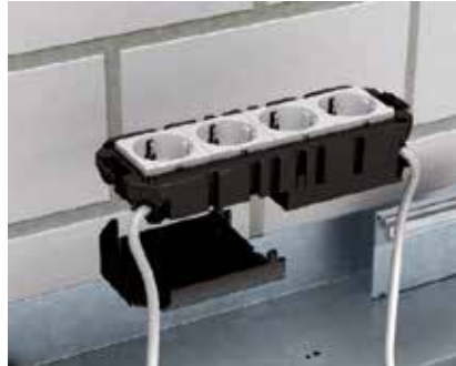
Socket mounting in module support Connect the connection cable to the socket and cover it with the protective housing. Safety: Use a protective housing.
